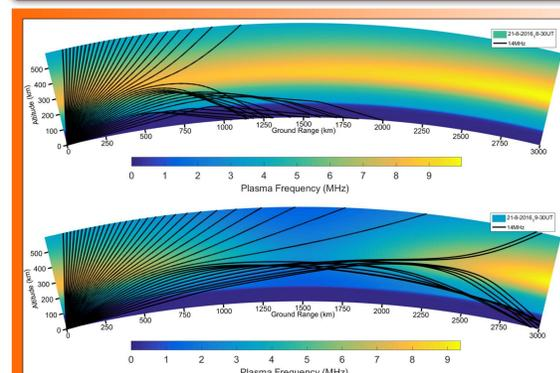
Figure 1. Raytrace on 14MHz ray through unperturbed ionosphere (top) and through eclipsed ionosphere (bottom)
