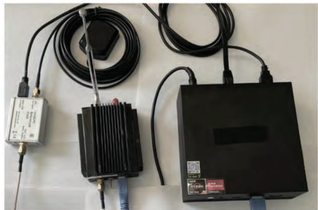
Figure 2 — The connections and basic layout of the HamSCI PSWS System. The core of the PSWS is the RX-888/KA9Q-radio WSPRDaemon-GRAPe HF SDR.
