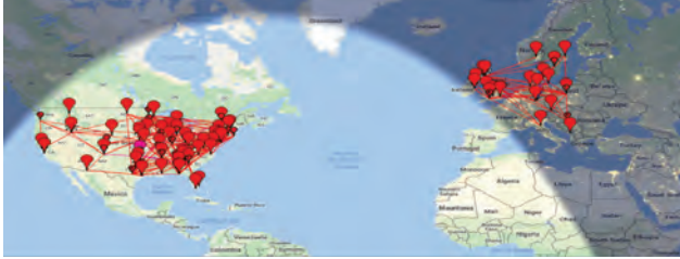
Figure 3 — PSK Reporter map illustrating MSK144 reports across the US and Europe ( pskreporter.info/pskmap ).
