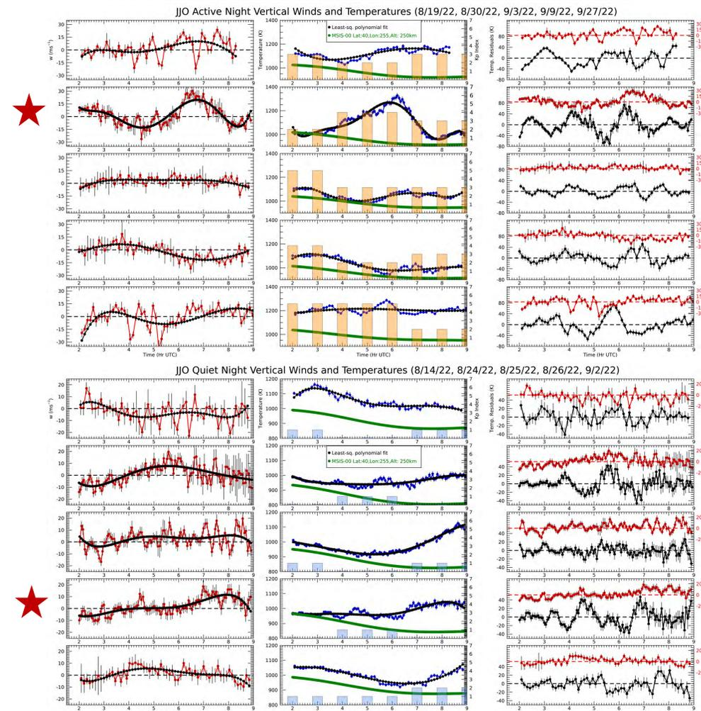
Figure 2: Observations from geomagnetically quiet (bottom) and active (top) conditions. Comparison of vertical winds (red) and temperature residuals (right, black) measured by HODI derived from the subtraction of observed temperatures (middle, blue) and a least-square polynomial fitting (middle, black). Temperatures are plotted with the NRLMSIS-00 empirical model (middle, green) and approximate kp index (bar graph).
