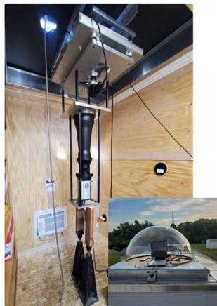
The Hot Oxygen Doppler Imager (HODI; pictured in Figure 1) is a 15 cm aperture Fabry-Perot Interferometer (FPI) comprised of 2 parallel, flat mirrors which can measure optical light emissions (630 nm; OI) to track the wind velocities and direction at a particular altitude of our atmosphere via Doppler shifts and widths.
