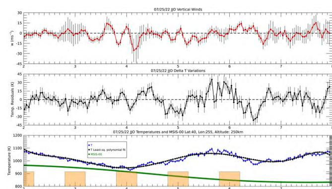
Figure 3: Potential GW event on 7/25/2022 between 03:00-04:00 UTC shown in vertical winds (top) and compared to temperature residuals (middle) derived from the subtraction of raw temperatures (bottom, blue) and a least-square polynomial fitting (bottom, black). Temperatures are plotted with approximate kp index (bar graph) and NRLMSIS-00 empirical model (bottom, green).
