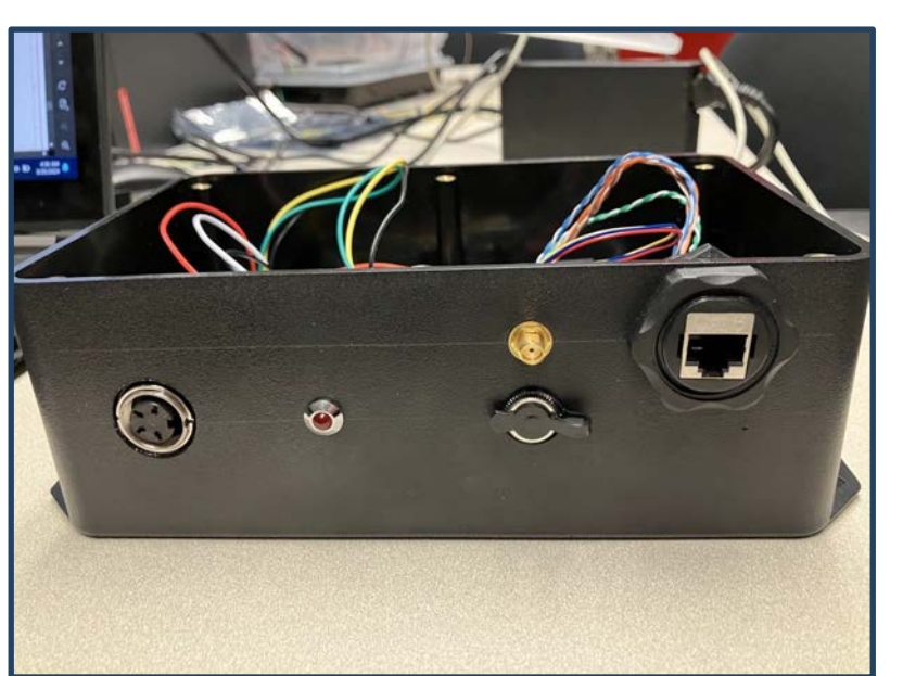
The device enclosure with the top case removed. Designed to be placed indoors, it has 4 jacks: sensor peripheral, DC power, GPS antenna coax, and Ethernet. A red indicator LED flashes when the device is on and logging data.
