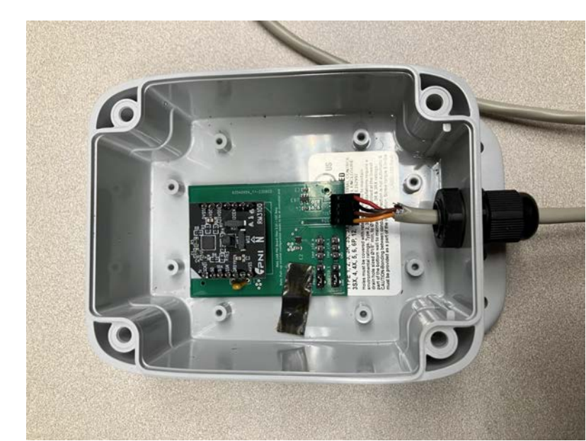
The sensor peripheral enclosure with the top removed—the sensors inside are a PNI rm3100 magnetometer and a TMP461 temperature sensor. The enclosure is NEMA 4X waterproof rated, and the shielded cable can be extended up to 100ft.
