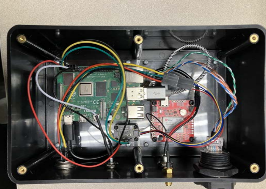
Shown above are 3 main electronic components: the GPS board, I2C active terminator, and Raspberry Pi computer. All of them are mounted on standoffs to an acrylic base plate manufactured in-house.
